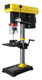
Drill presses are generally electrically powered and can be either hardwired into the electrical circuit or plugged into an electrical outlet. The switch to turn on/off the drill press are generally located for easy access by the operator.
