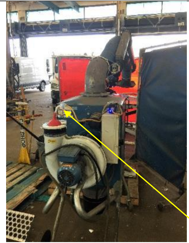
Portable LEV Filtered Exhaust Sample
