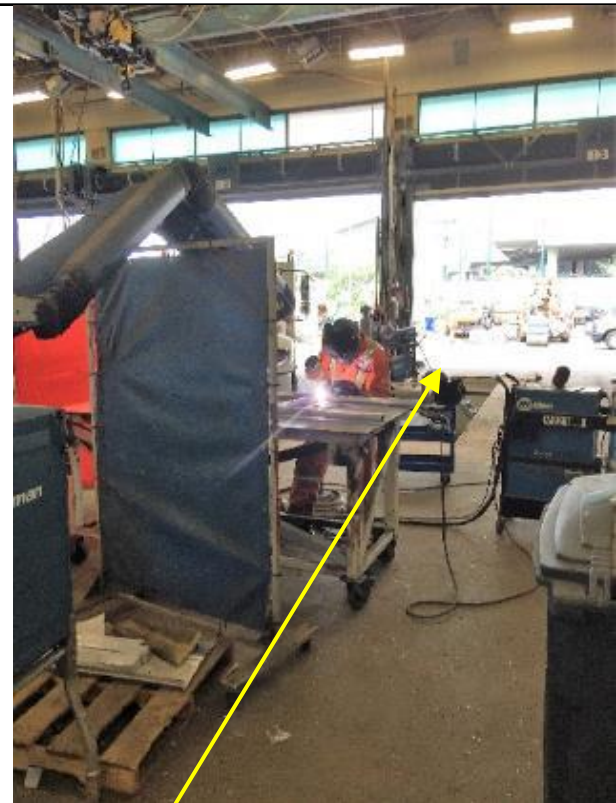
Personal Sample -Aluminum Welding with LEV
